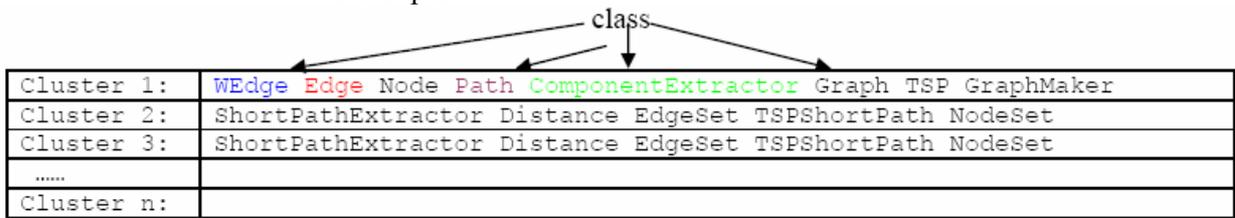
For example Cluster1(component1) contains classes{Wedge, Edge, Node, Path,...}
